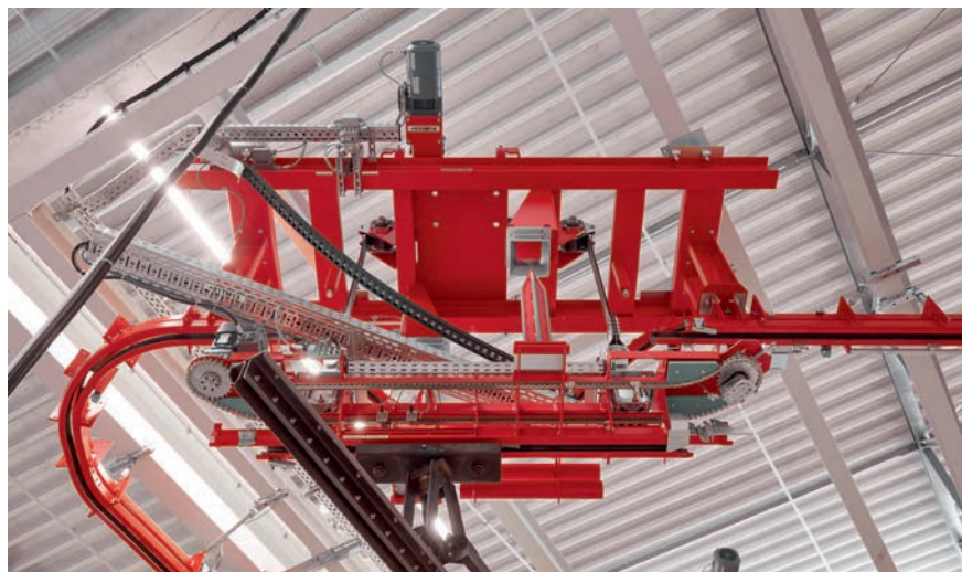
Lifting and lowering stations for the long load bars with two parallel, non-guided belt lifters.
