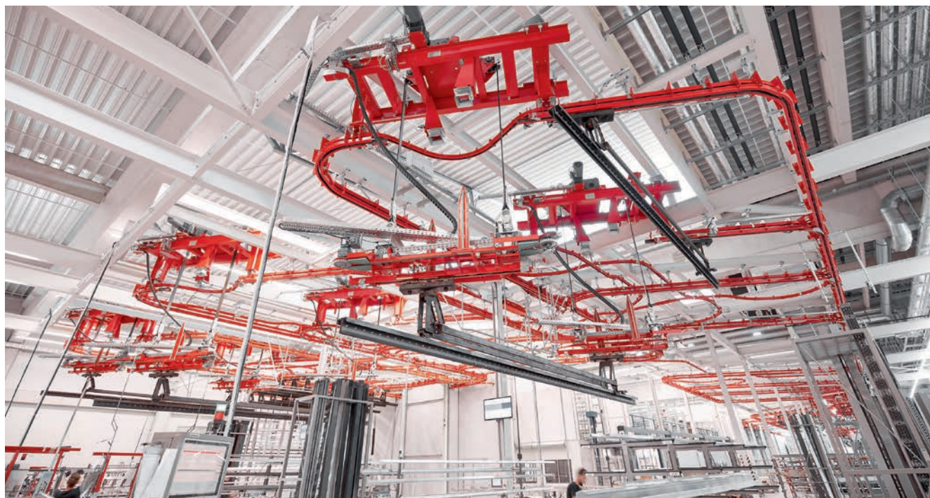
The compact design of the new power-and-free system at Solarlux allows it to operate in a very small space
